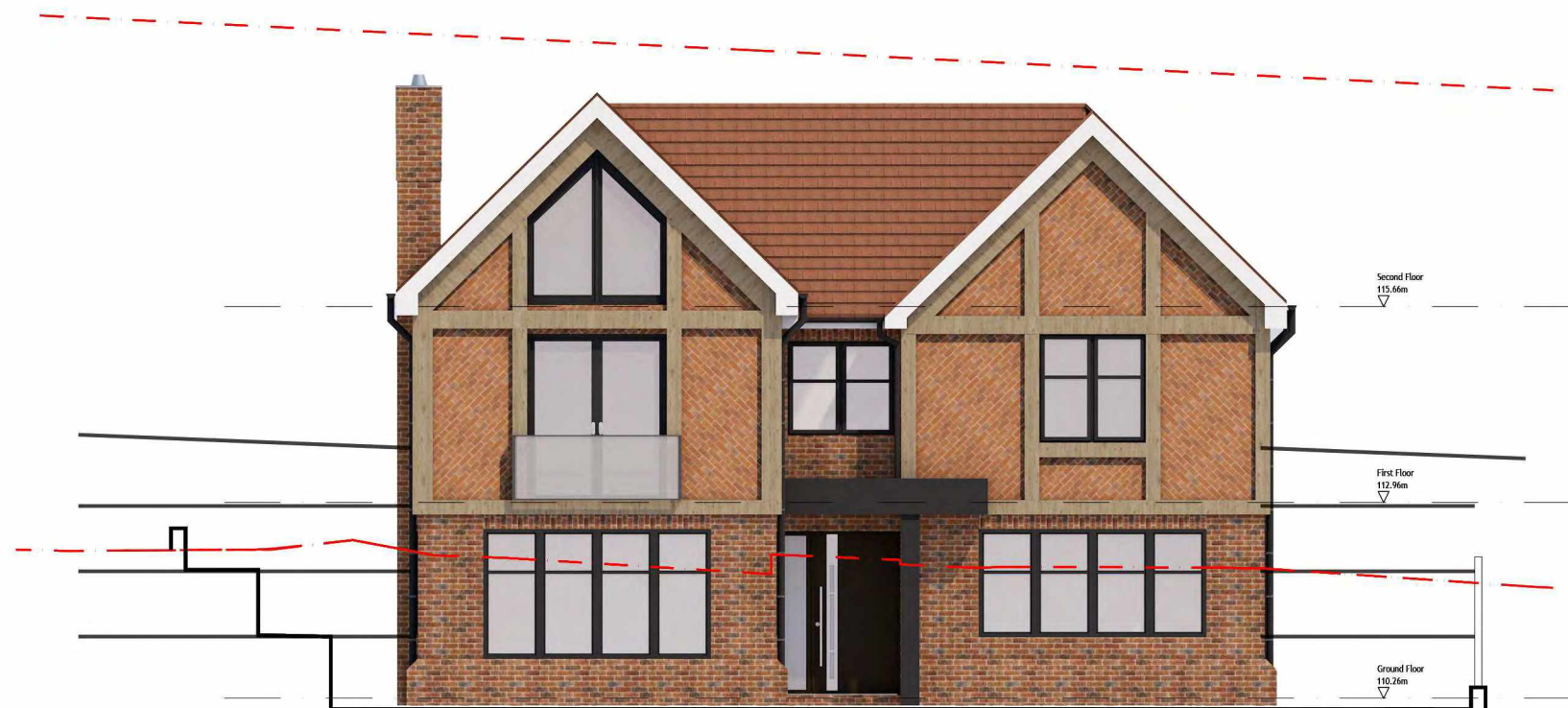
Proposed West Elevation (Frontage) Unit 1
